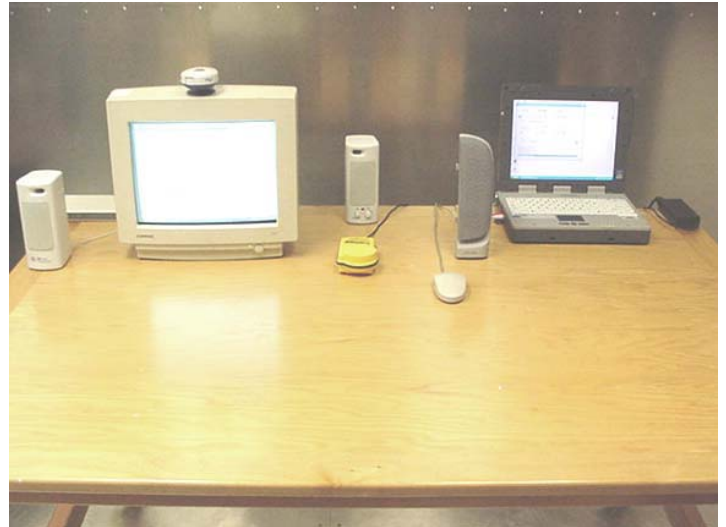
Photograph H-2 – AC Powerline Conducted Emission Cable Placement
