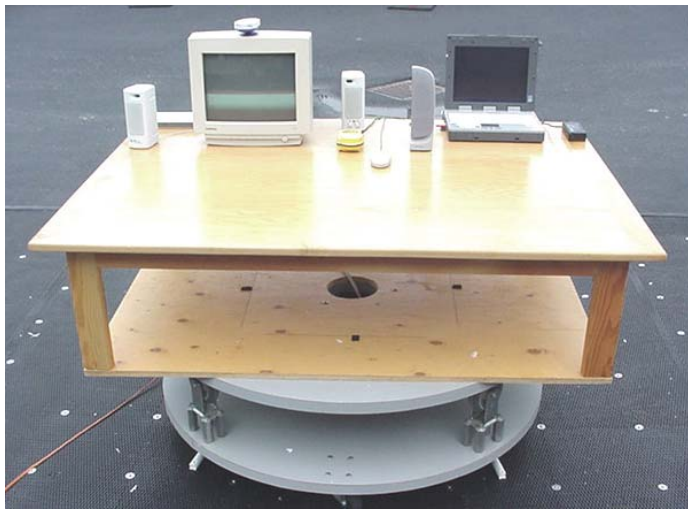
Photograph E-3 - Front of Radiated Emission Configuration
