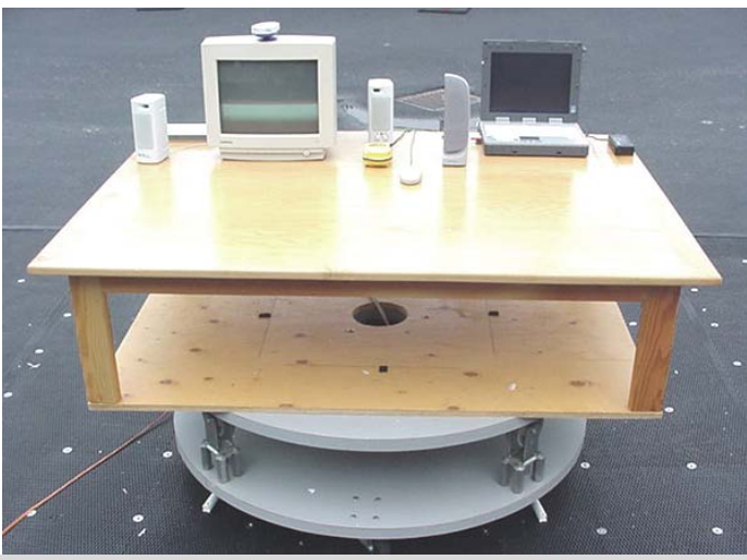
Photograph F-3 - Front of Radiated Emission Configuration
