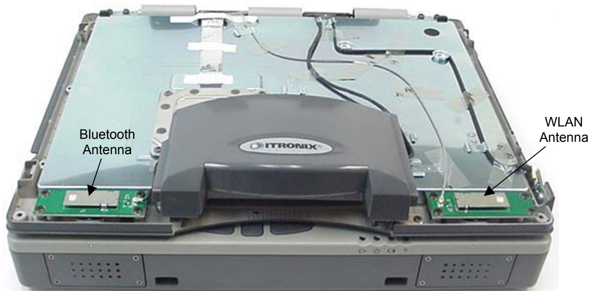
Photograph A-7 – Surface Mount Antenna Placement
