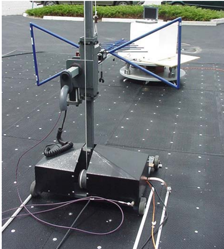
DUT Cellular Band with Bilog receive antenna
