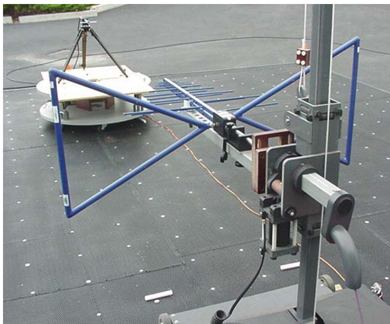
Dipole Substitution antenna
