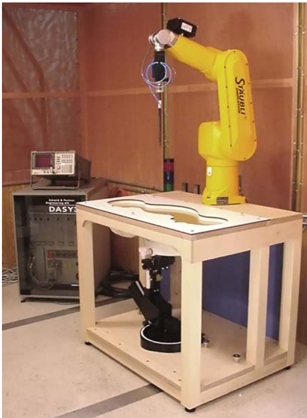
DASY3 SAR Measurement System with SAM phantom
