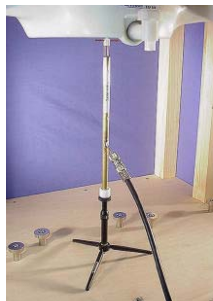
2450MHz System Check Setup Photograph
