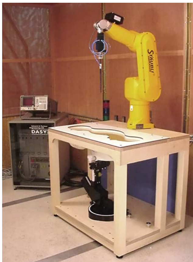
DASY3 SAR Measurement System with SAM phantom
