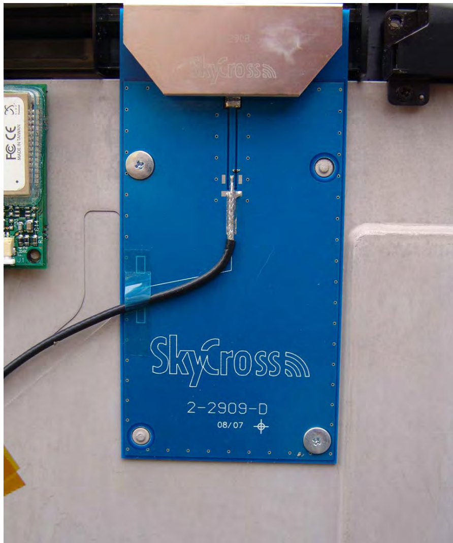
Co-Located WLAN, Inverted F antenna left and right
