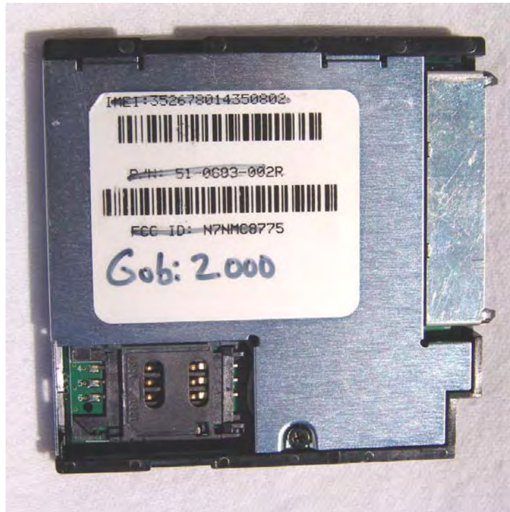
IX-GOB12 CRMA module bottom view
