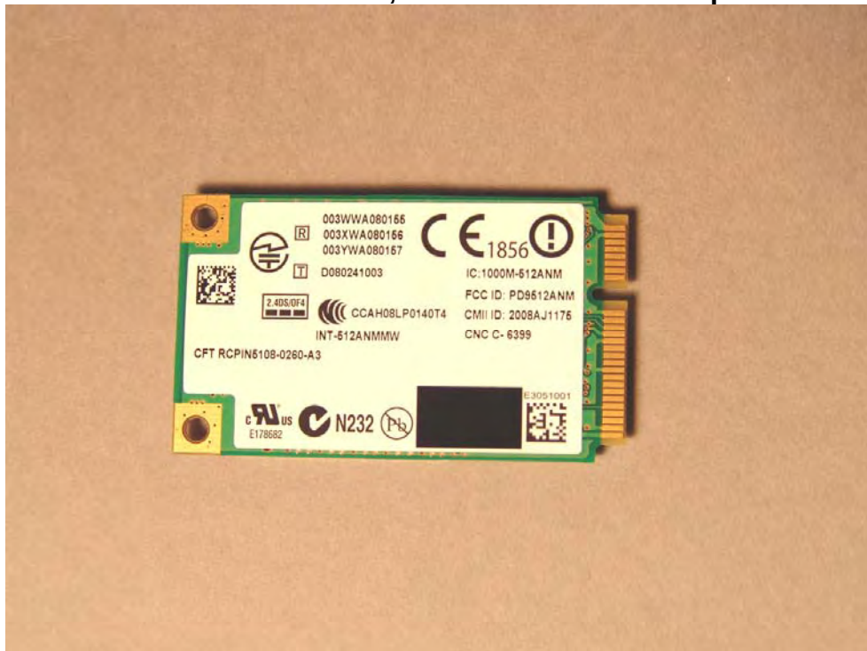
Bottom side of WLAN, OEM Identifier label in place
