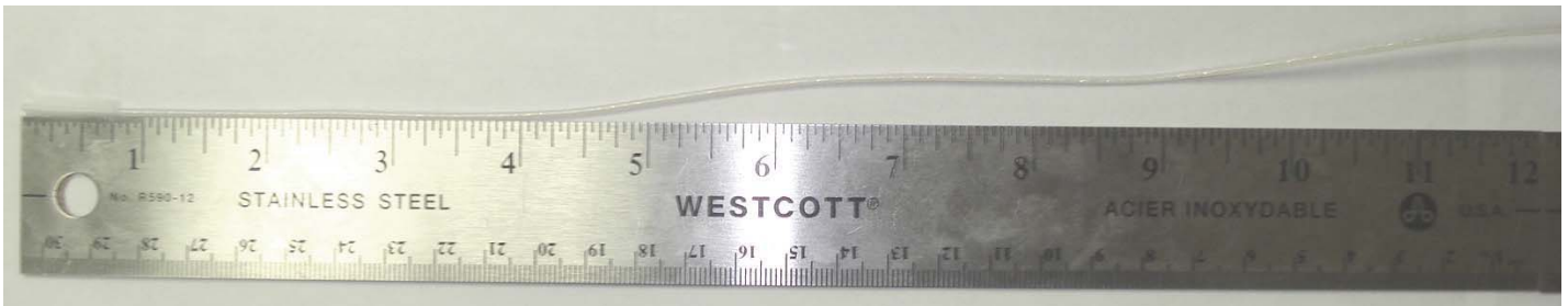
DUT with Wire Antenna (162-174 MHz) and Wire Microphone audio accessory
