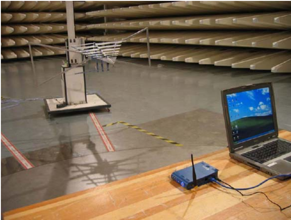
Radiated Emissions Test Setup
