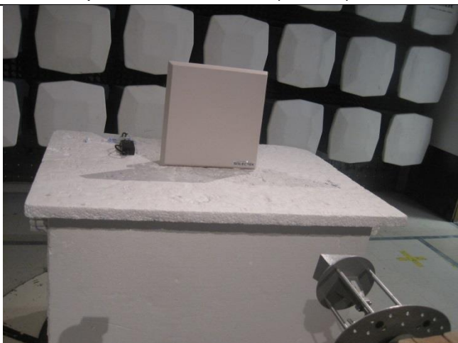
Radiated Spurious Emissions 18-40GHz (23dBi Ant) – Front View
