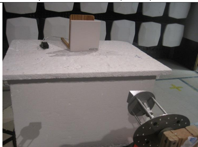
Radiated Spurious Emissions 18-40GHz (20dBi Ant) – Front View
