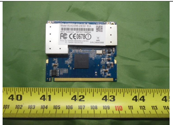
EUT – RF Module with Shielding Top View
