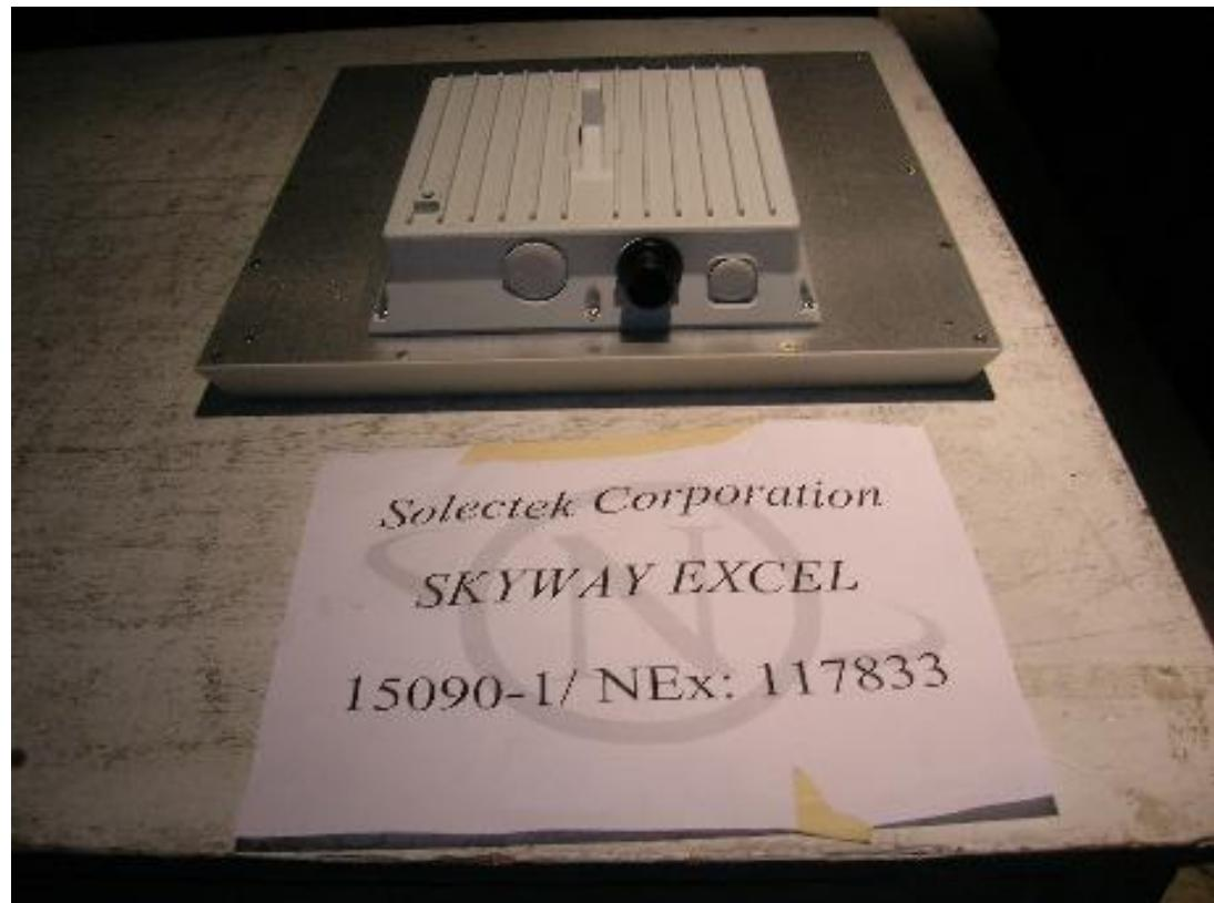
Components of system: Radio, POE, POE power adapter. Indoor Unshielded cables used for checking out the system, Yellow Ethernet to be replaced at installation with Outdoor Shielded Ethernet. Radio may have three antennas: 2 port Planar, 2 port parabolic and 3 port omni. Plastic insert to left of Ethernet cable can be configured with third RF Port.
