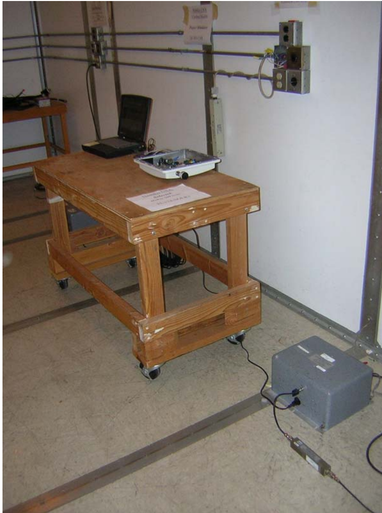
Photograph 1. Conducted Emissions Test Configuration
