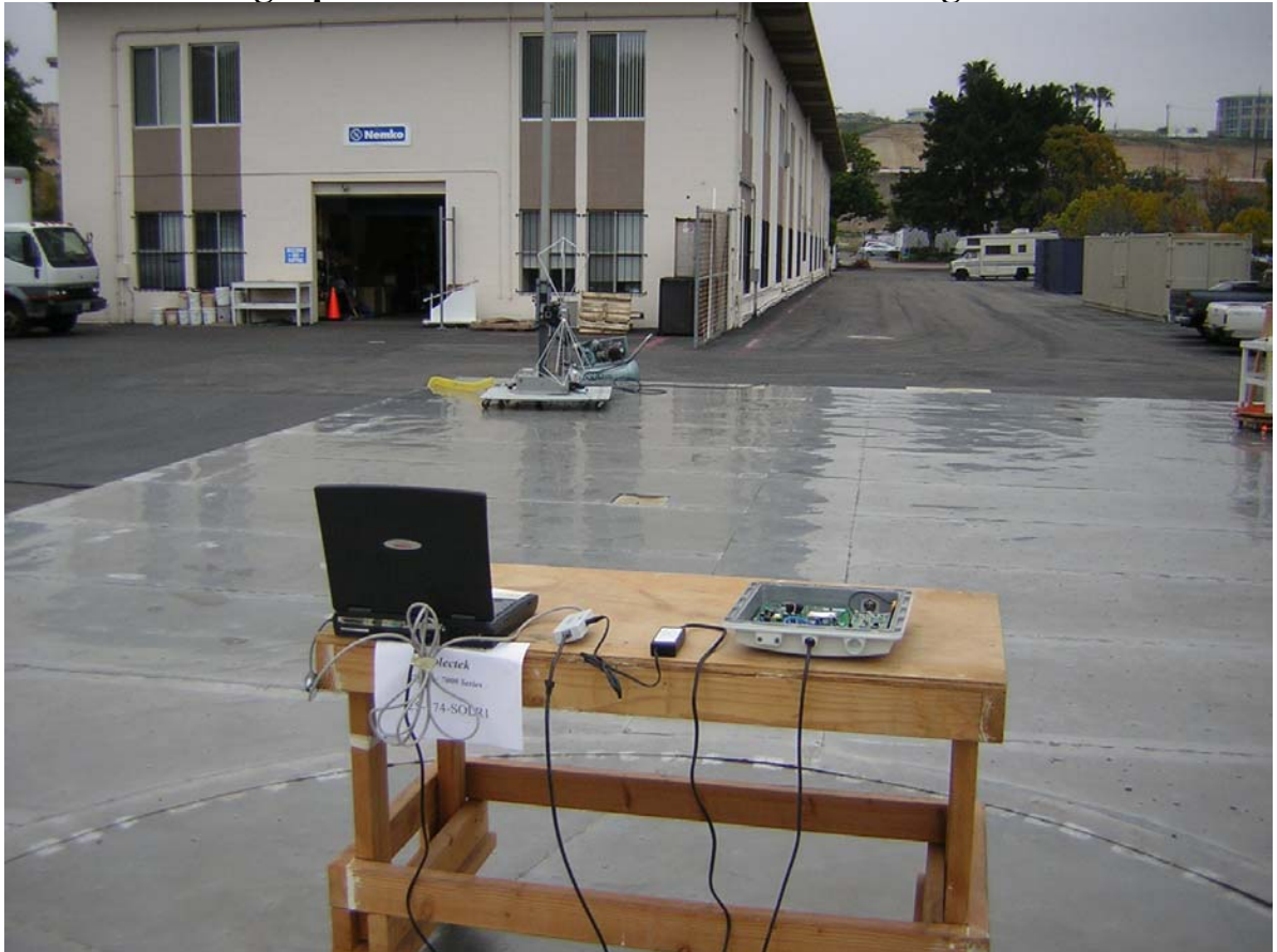
Photograph 2. Radiated Emissions Test Configuration
