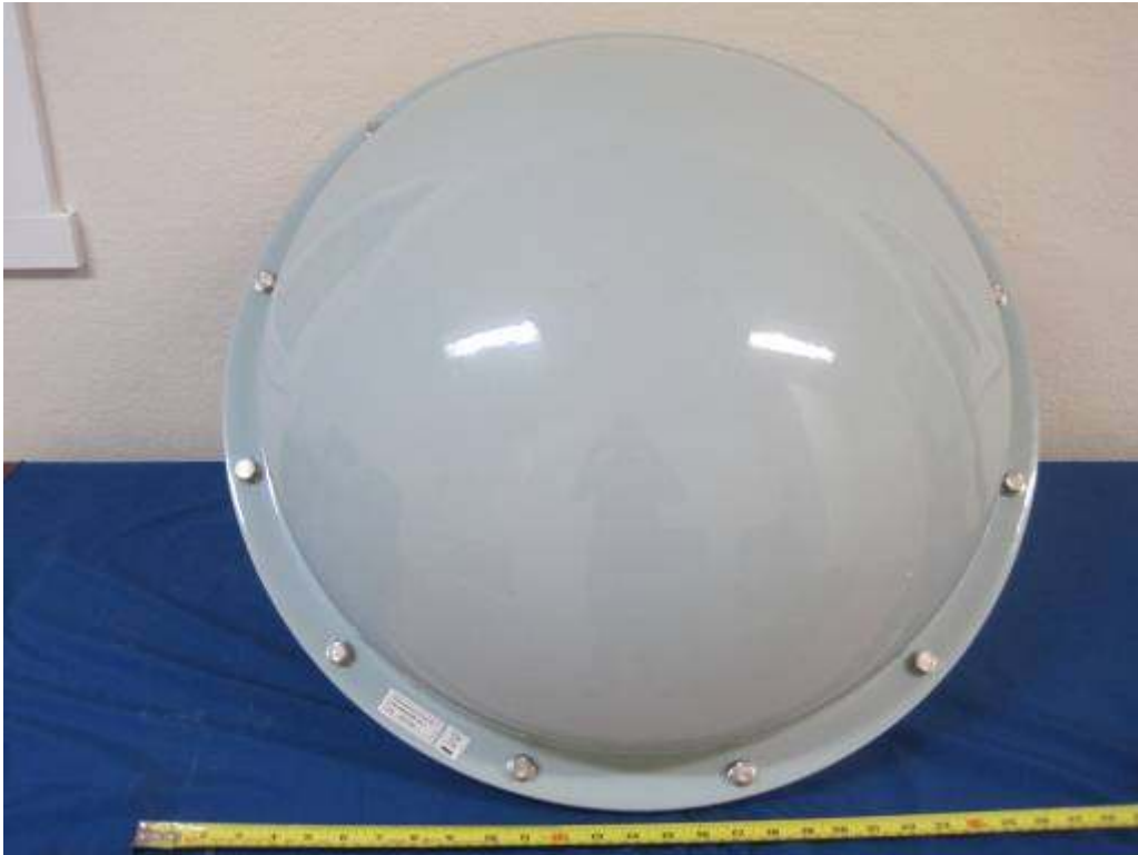
Antenna: External Antenna with 29dBi gain
