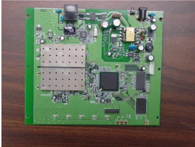
Photo 3: PCB1 top with shield
