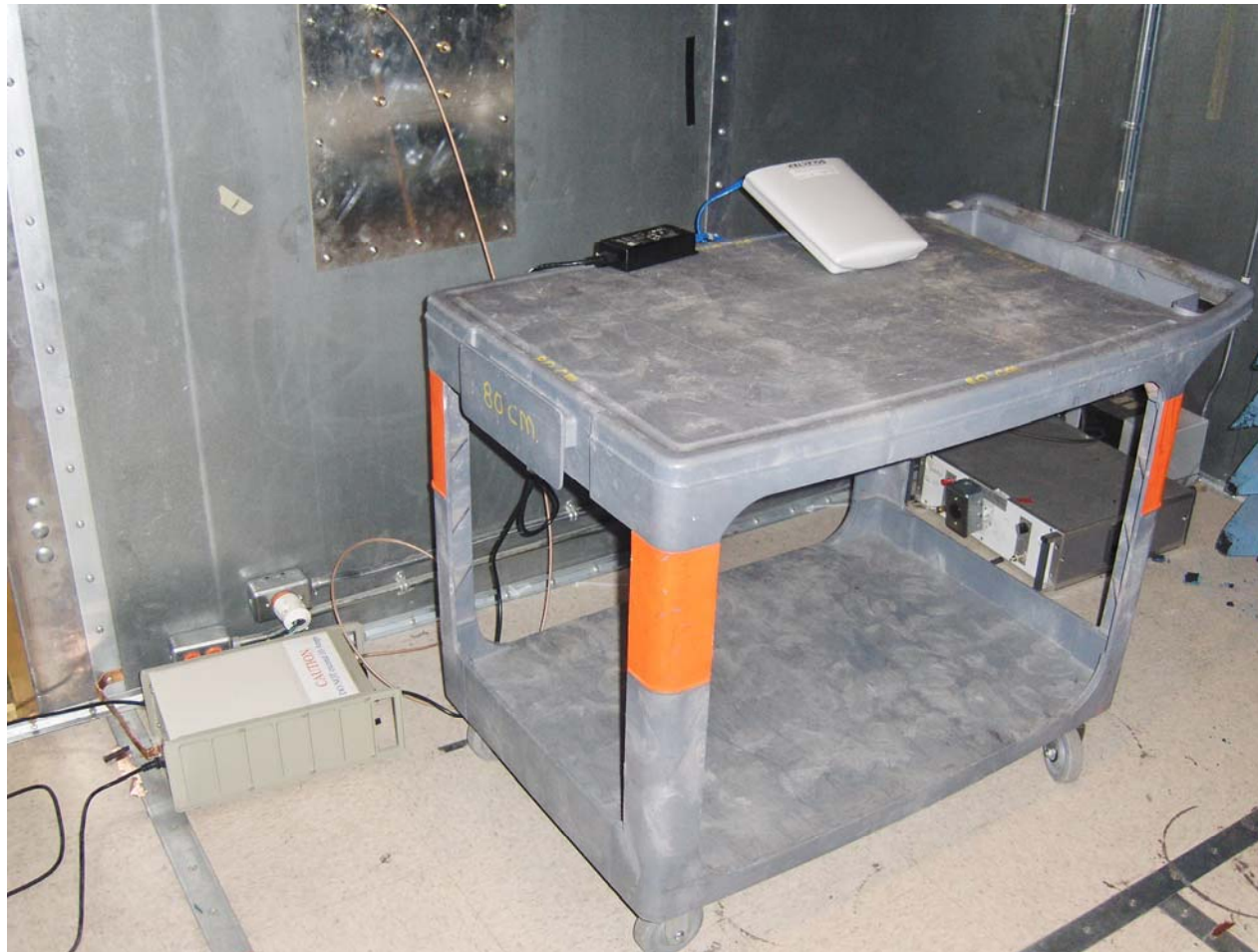
Plot #2: Test setup for AC Conducted Emissions
