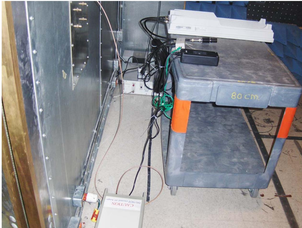
Plot #2: Test setup for AC Conducted Emissions
