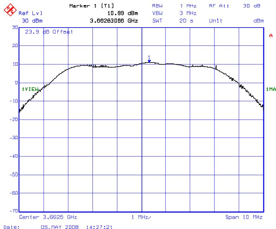
**Plot # 2(b): Peak Conducted Power Density Measurement wrt. 18.5 dBi Gain (Minimum) Antenna
