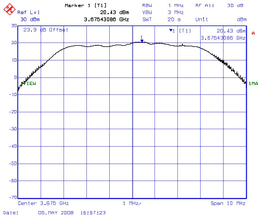
Plot # 2(a): Peak Conducted Power Density Measurement wrt. 18.5 dBi Gain (Minimum) Antenna
