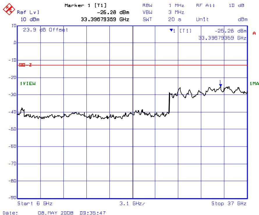
**Plot # 9(a): Transmitter Conducted Spurious Emissions**
