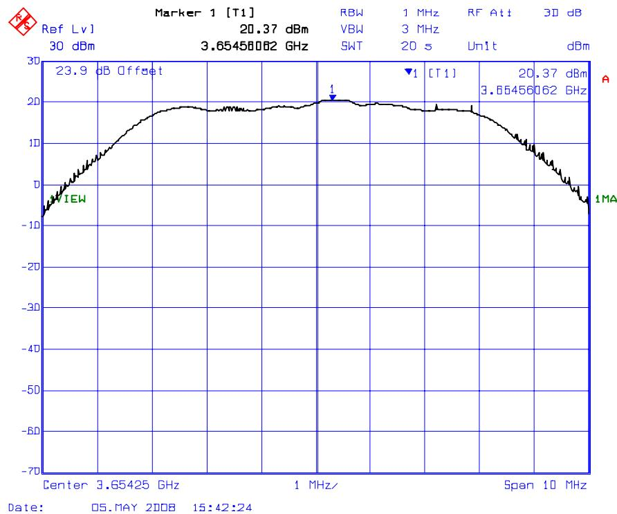
**Plot # 1(b): Peak Conducted Power Density Measurement wrt. 9 dBi Gain (Minimum) Antenna (Maximum Power Setting: 19 dBm)**
