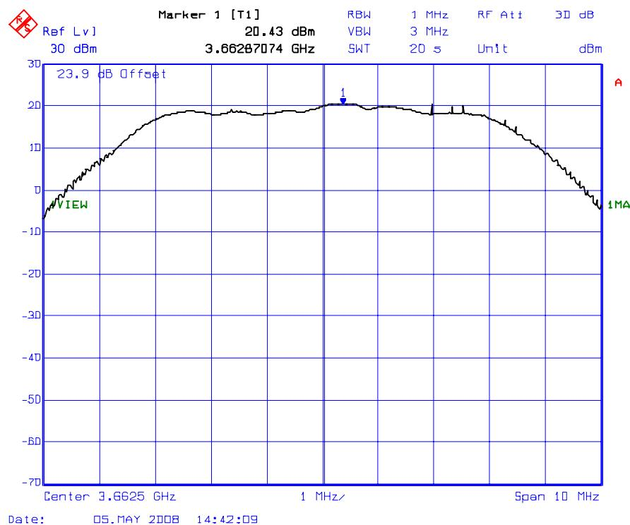
Plot # 1(b): Peak Conducted Power Density Measurement wrt. 9 dBi Gain (Minimum) Antenna
