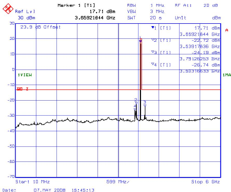
**Plot # 8(b): Transmitter Conducted Spurious Emissions**
