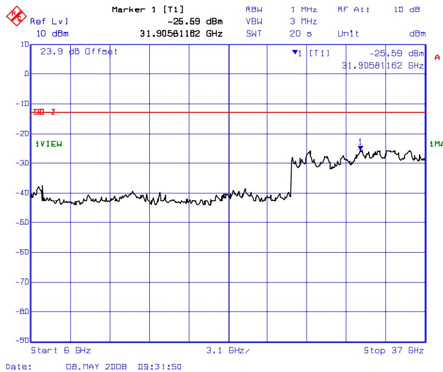
**Plot # 8(a): Transmitter Conducted Spurious Emissions**
