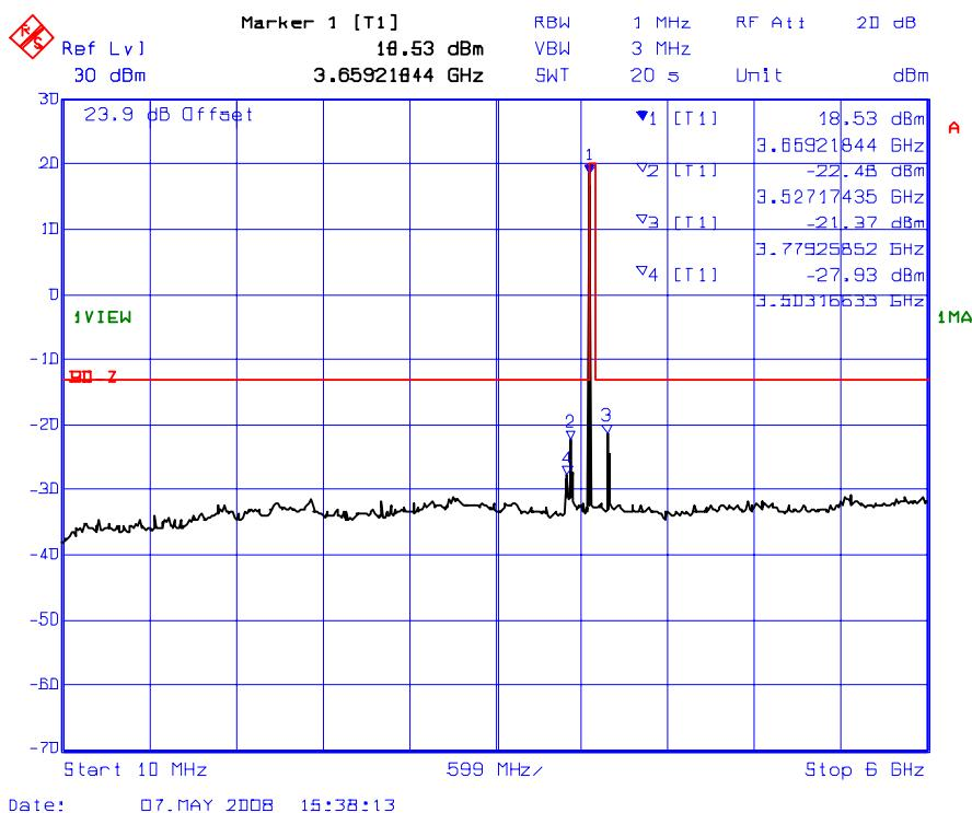
**Plot # 7(b): Transmitter Conducted Spurious Emissions**
