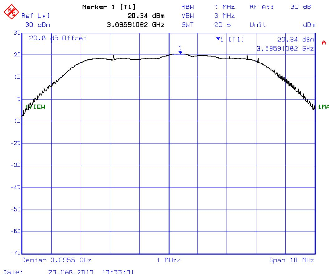
Plot # 1(b): Peak Conducted Power Density Measurement wrt. 18.5 dBi Gain (Minimum) Antenna
