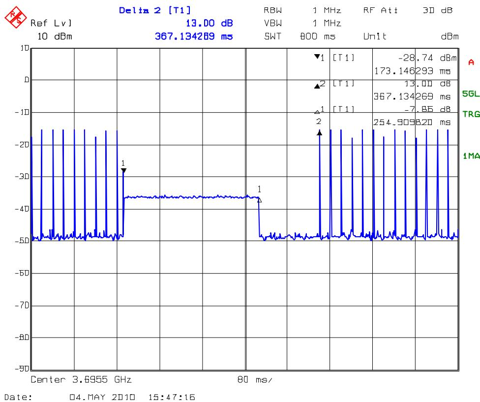
Note: The above plot shows that Tx turns OFF when an interference signal was applied to the EUT and turns ON when the interference signal was removed.
