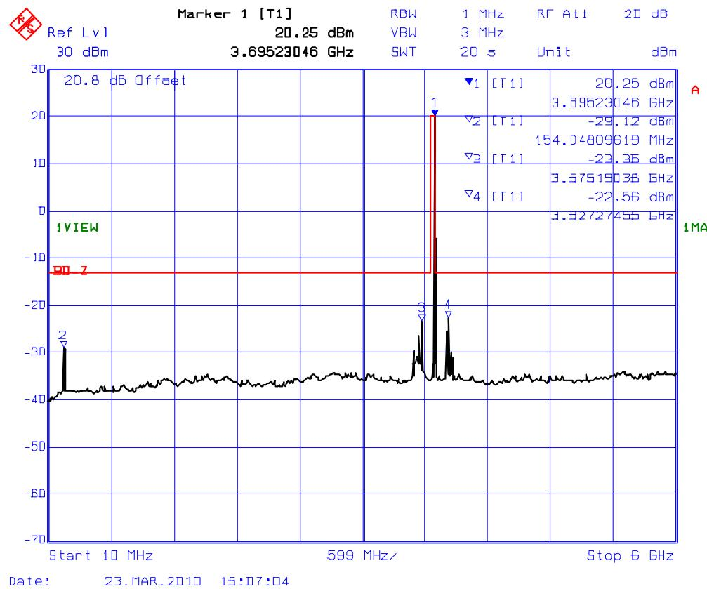
**Plot # 4(b): Transmitter Conducted Spurious Emissions**
