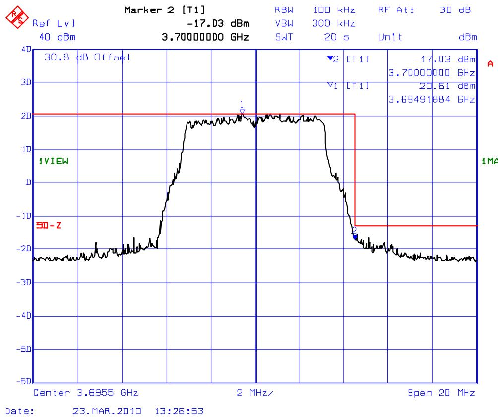
**Plot # 4(a): Transmitter Conducted Spurious Emissions**
