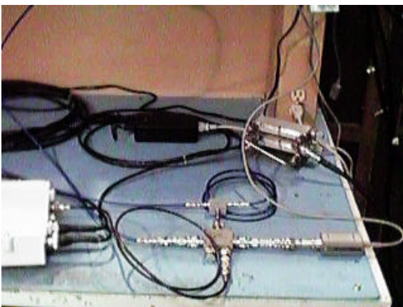
Figure 5 - Setup of attenuators, splitter, and combiner
