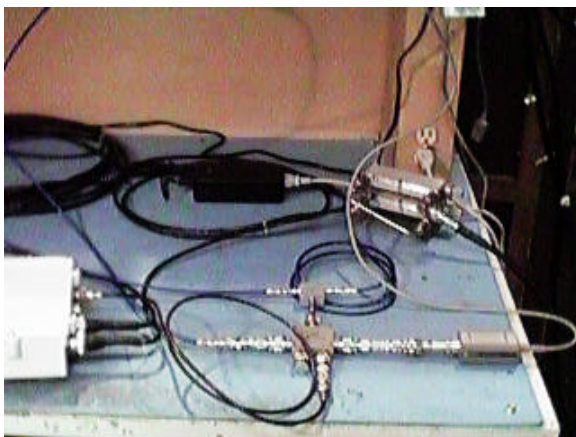
Figure 5 - Setup of attenuators, splitter, and combiner
