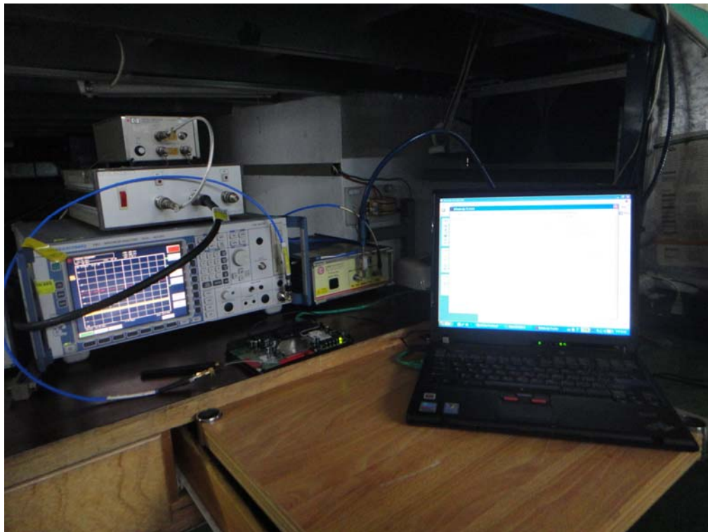
ANTENNA PORT CONDUCTED RF MEASUREMENT SETUP
