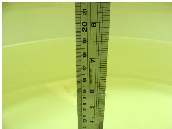
Fig 6.2 Photo of Liquid Height for Body SAR
