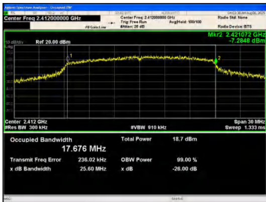
IEEE 802.11n_Channel 1_20MHz_Antenna 0
