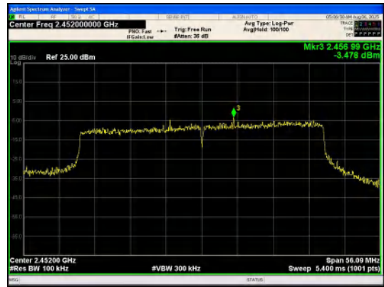
In-Band Reference Level IEEE 802.11ax_Channel 9_40MHz_Antenna 0_RU&Index SU
