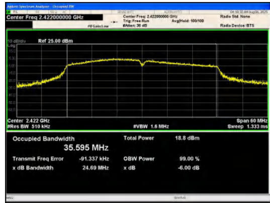
IEEE 802.11n_Channel 3_40MHz_Antenna 0
