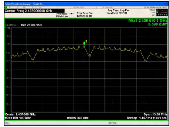
In-Band Reference Level IEEE 802.11b_Channel 6_20MHz_Antenna 0
