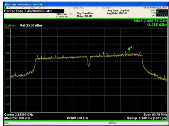
In-Band Reference Level IEEE 802.11n_Channel 9_40MHz_Antenna 0
