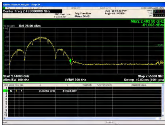
Out Of Band Emission IEEE 802.11b_Channel 11_20MHz_Antenna 0
