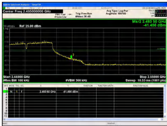
Out Of Band Emission IEEE 802.11n_Channel 9_40MHz_Antenna 0
