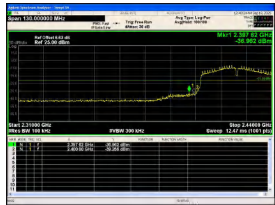
Out Of Band Emission IEEE 802.11n_Channel 3_40MHz_Antenna 0
