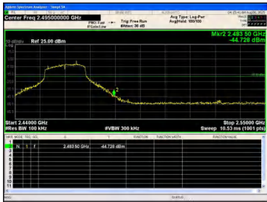
Out Of Band Emission IEEE 802.11n_Channel 11_20MHz_Antenna 0
