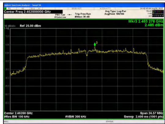
In-Band Reference Level IEEE 802.11ax_Channel 11_20MHz_Antenna 0_RU&Index SU
