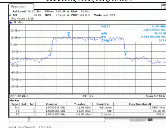
26%OBW Band 2 3MHz/1880.0/Mid 16QAM 15@0
