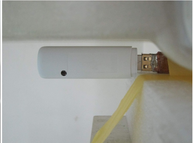
USB Cable Plug-in for USB Configuration 4 Vertical Back with Phantom 0.5 cm Gap
