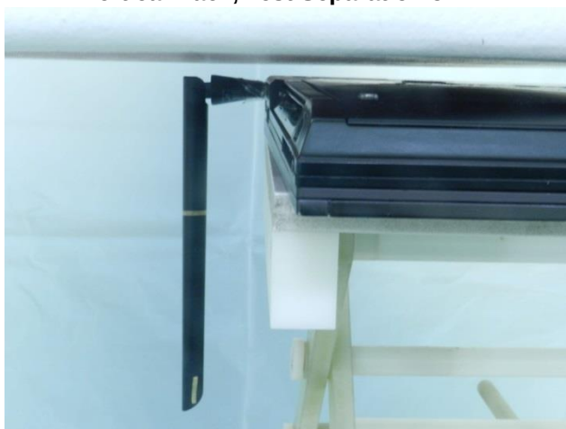
Tip Mode, Test Separation 5 mm(Configuration 2)
