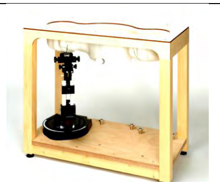
Fig 5.8 Photo of SAM Phantom
