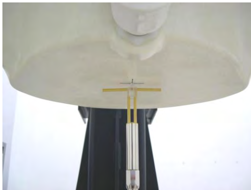
Fig 7.2 Photo of Dipole Setup
