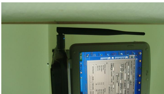
Direct Laptop Plug-in for USB Configuration 5 (Tip Mode with Phantom 5 mm Gap and Antenna Status 90 °)
