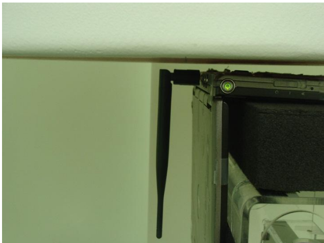
Direct Laptop Plug-in for USB Configuration 1 (Horizontal Up with Phantom 5 mm Gap and Antenna Status 90 °)
