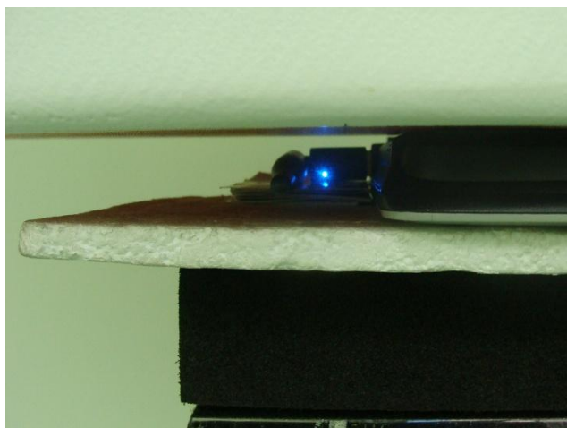
Direct Laptop Plug-in for USB Configuration 4 (Vertical Back with Phantom 5 mm Gap and Antenna Status 90 °)
