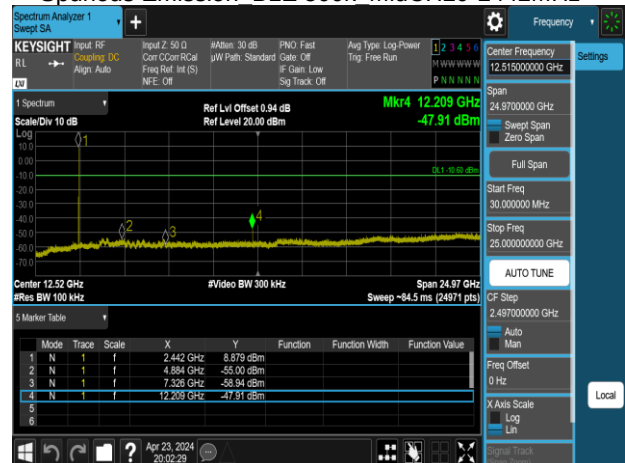
Spurious Emission BLE 500k HighCH39-2480MHz
