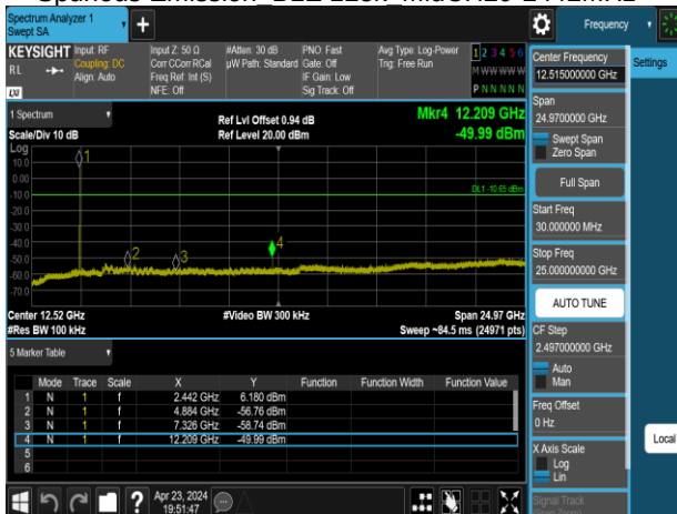
Spurious Emission BLE 125k HighCH39-2480MHz
