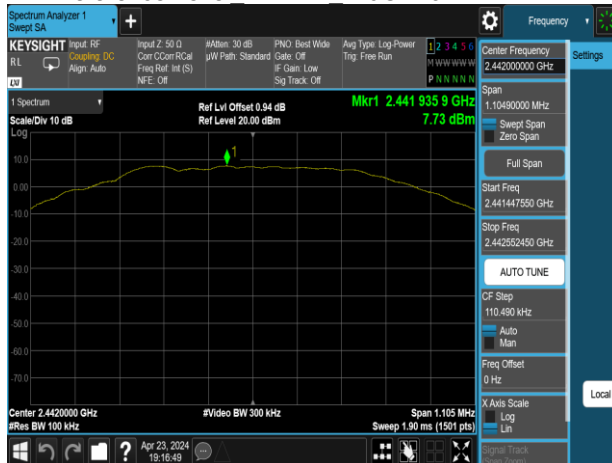
Reference Level BLE 1M HighCH39-2480MHz
