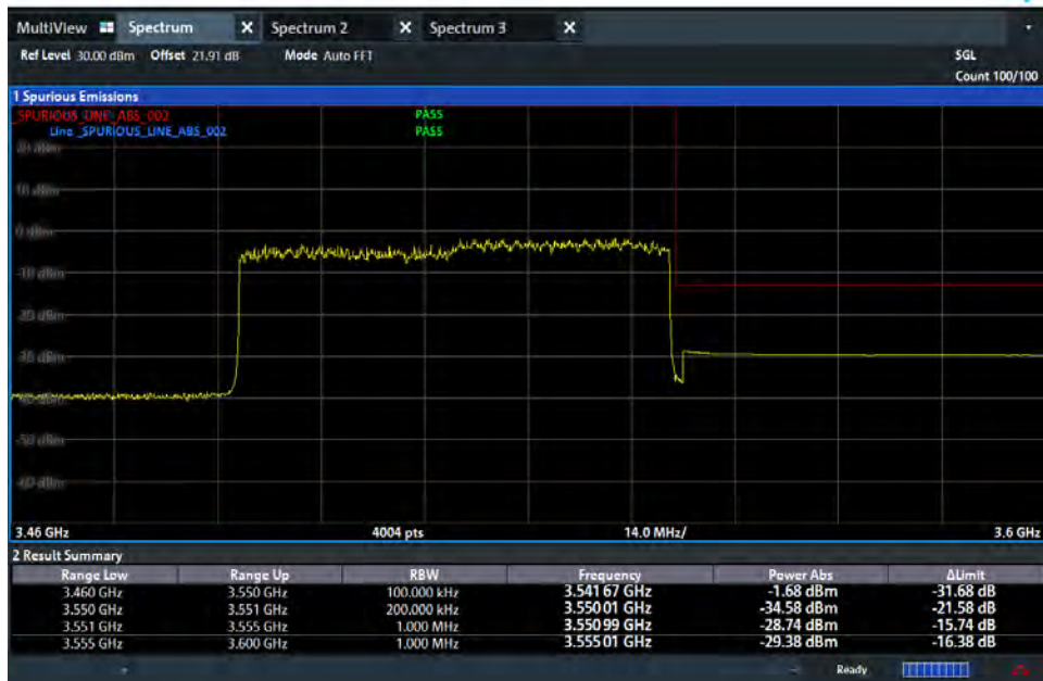
BE_n77_60M_High CH_DL634666_3519.99MHz_DFT_QPSK_Full RB
