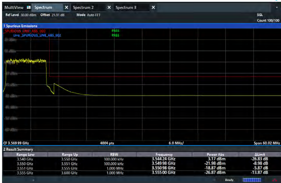
BE_n77_10M_High CH_DL636332_3544.98MHz_CP_QPSK_Full RB
