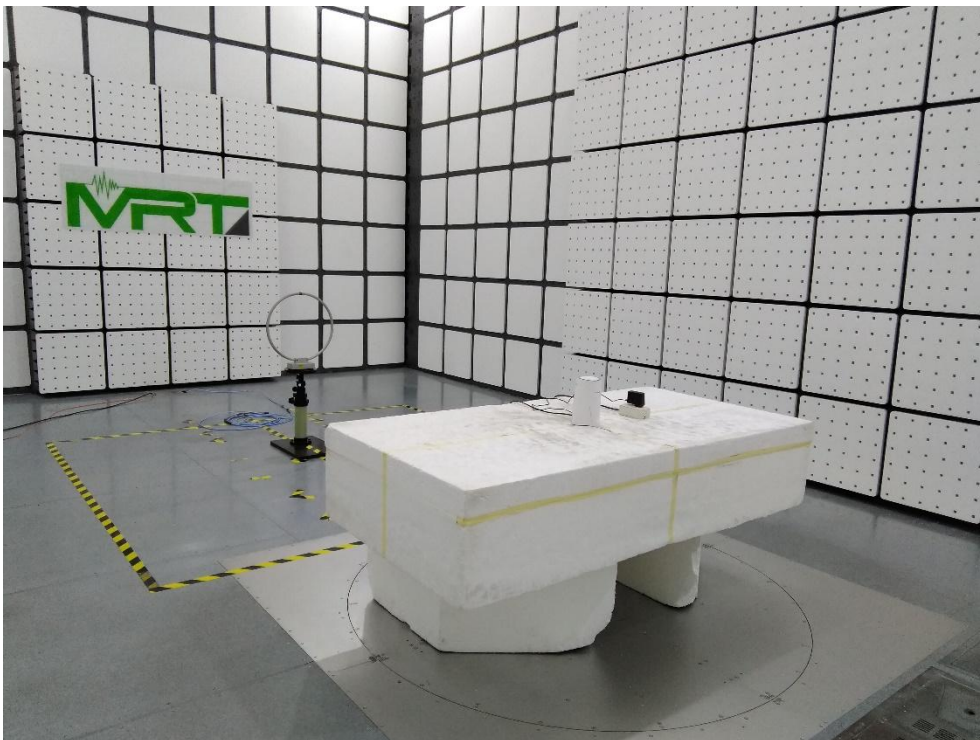
Description: Radiated Emission Test Setup for 9kHz~30MHz
