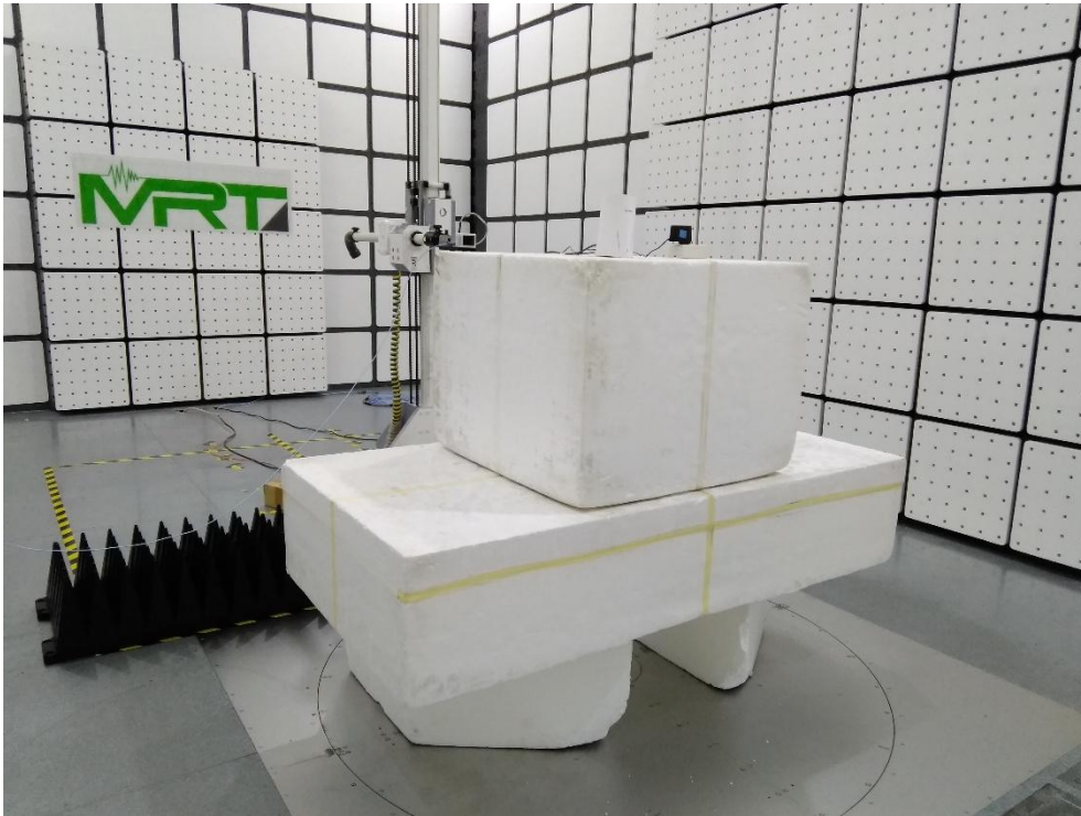
Description: Radiated Emission Test Setup for 9kHz~30MHz
