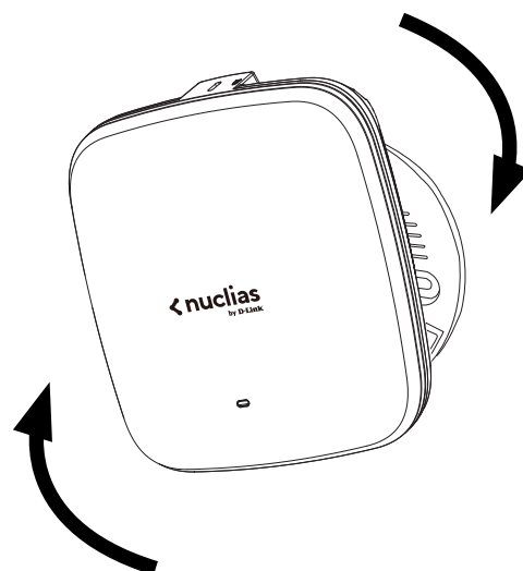
Figure 8: Placing The Access Point
