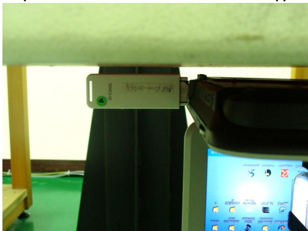
USB Configuration 4 (Vertical Back with Phantom 5 mm Gap)
