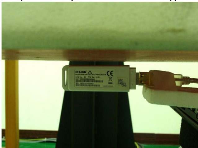
USB Configuration 3 (Vertical Front with Phantom 5 mm Gap)
