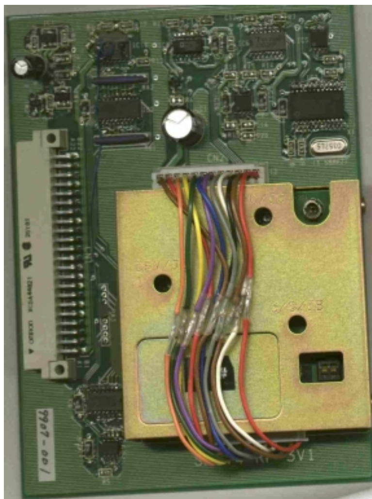
Interface board with Transmitter enclosed in metal box
