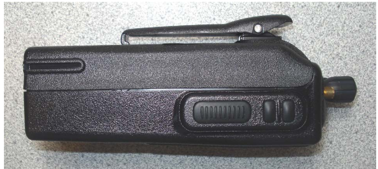
Left Side of Radio with Battery 'b' (3450 mAh) and Belt-Clip accessory
