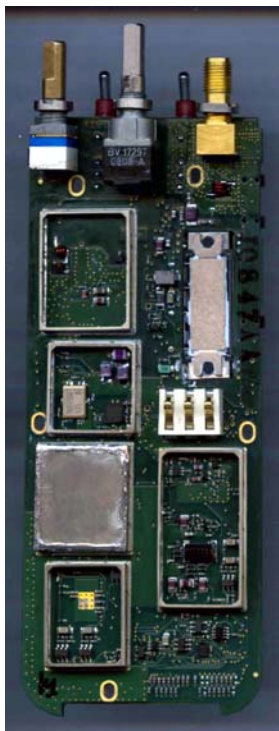
RF board bottom side.
