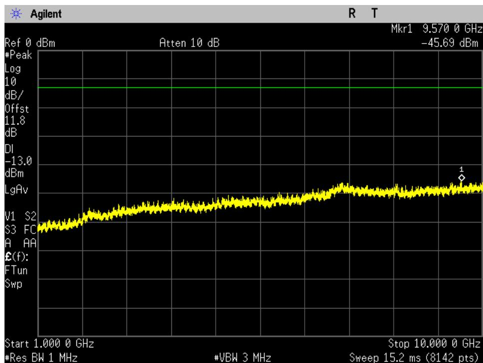
**Radiated Spurious\_VHF\_CW\_161.625 MHz\_30 - 1000 MHz**
