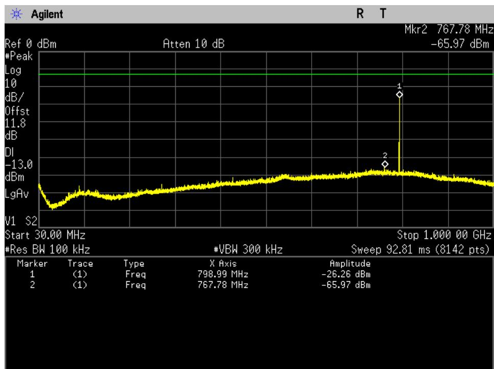
**Radiated Spurious\_700 band\_CW\_769.025 MHz\_1 - 10 GHz**
