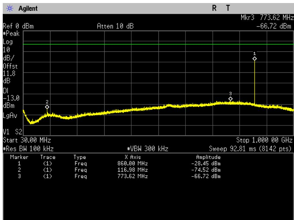
**Radiated Spurious\_800 band\_CW\_810.025 MHz\_1 - 10 GHz**
