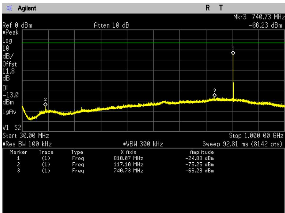
**Radiated Spurious\_800 band\_C4FM\_859.975 MHz\_1 - 10 GHz**
