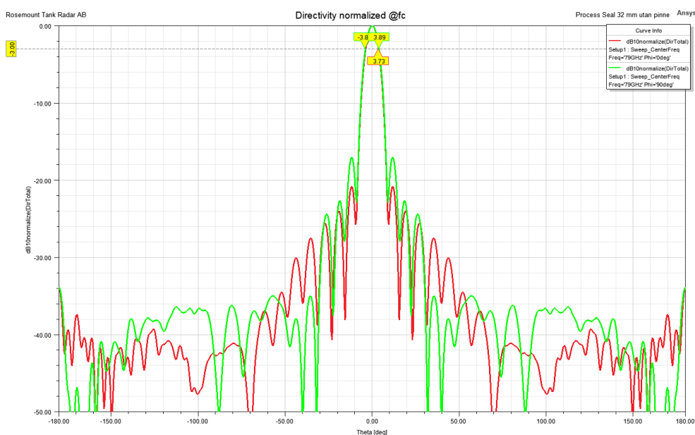
Normalized directivity for the Process Seal (29 mm) antenna @79 GHz
