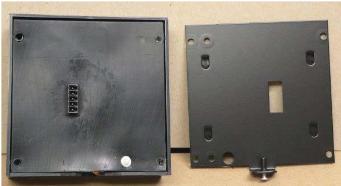
This is the rear view of the card reader with the metal back plate removed.
