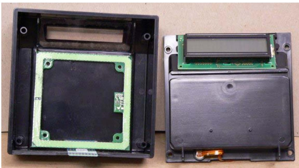
This is the inner shell removed and flipped over, showing the placement of the antenna.
