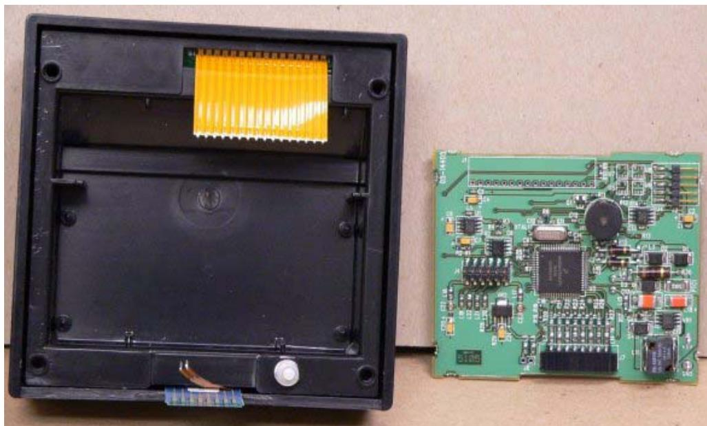
The printed circuit board rests in a bathtub shaped plastic inner shell.
