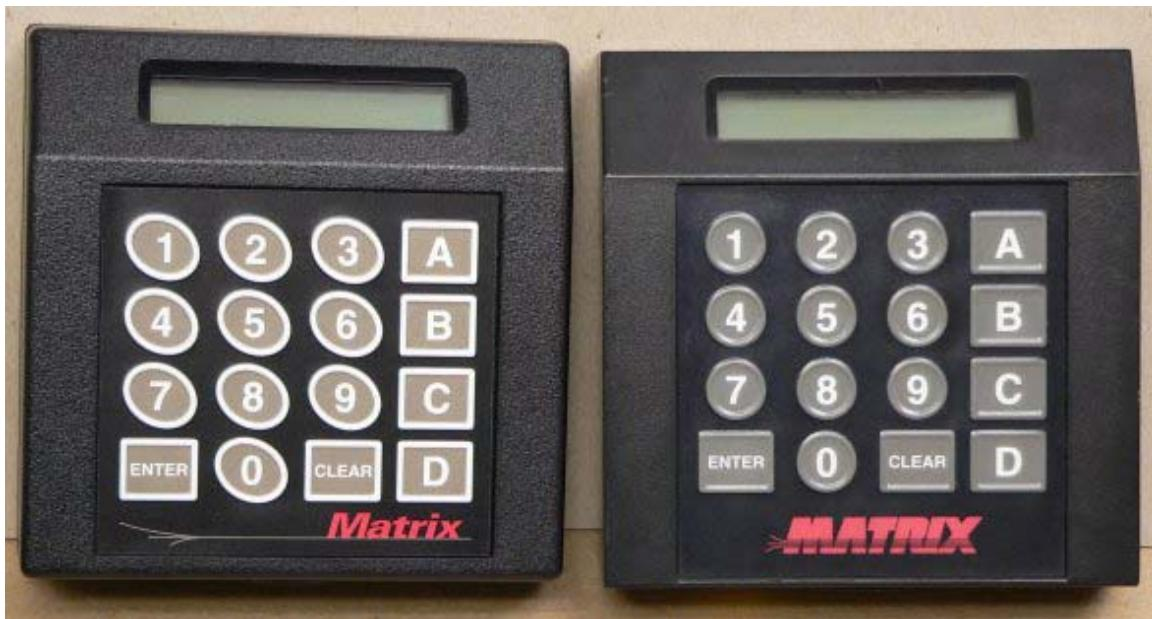
We are in the process of changing our company logo and the look of the card reader. The outer shell on the left has rounded edges and a deeper texture. Both shells are made of plastic so they will not affect the RF characteristics of the card reader. We may use either outer shell in production.
