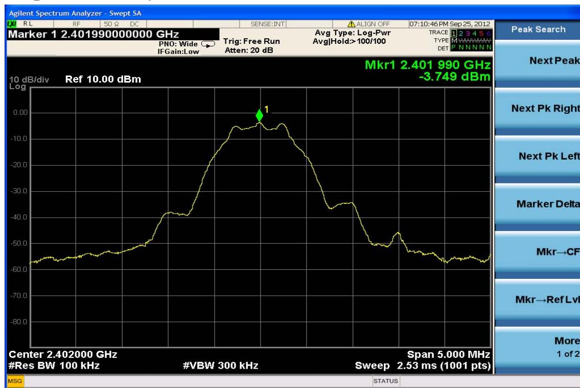
**Power Spectral Density Test Plot (CH-Mid)**
