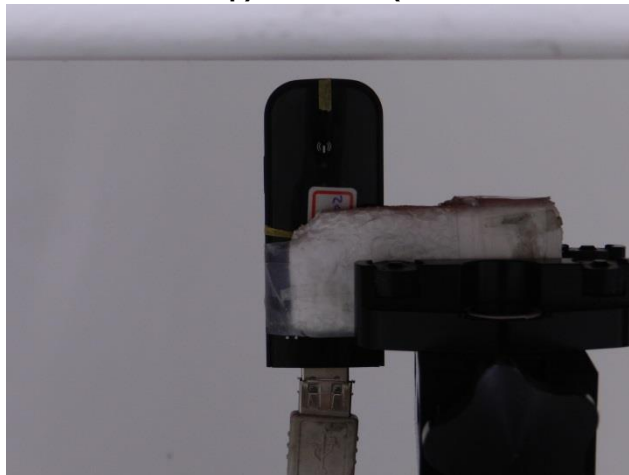
Direct Laptop Plug-in for USB Configuration 5 (Tip Mode with Phantom 5 mm Gap)
