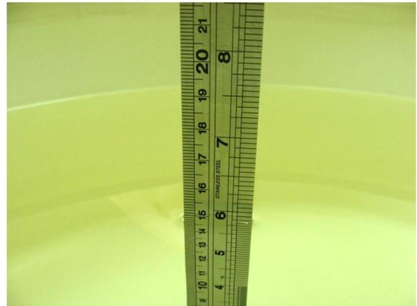
Fig 6.2 Photo of Liquid Height for Body SAR
