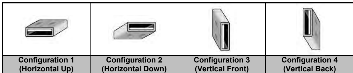
Fig 9.1 Illustration for USB Connector Orientations
