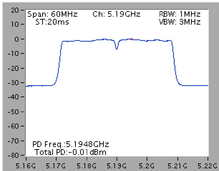
Power Density Plot on Configuration IEEE 802.11ac MCS0, Nss1 VHT 80MHz / Ant. 3+ Ant. 4+ Ant. 5 / 5210 MHz
