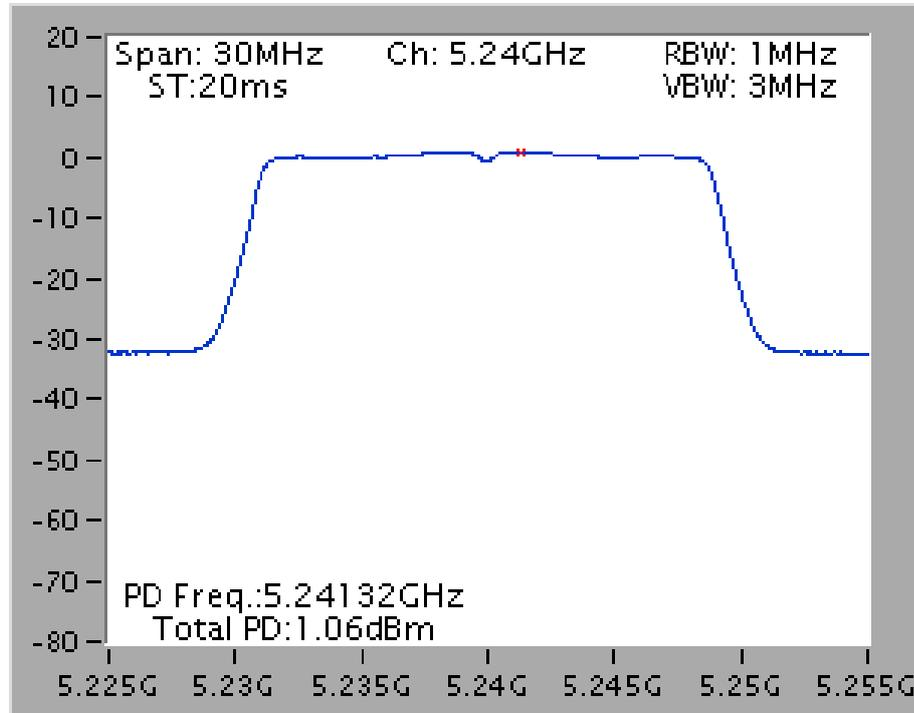
Power Density Plot on Configuration IEEE 802.11ac MCS0, Nss1 40MHz / Ant. 3+ Ant. 4+ Ant. 5 /
