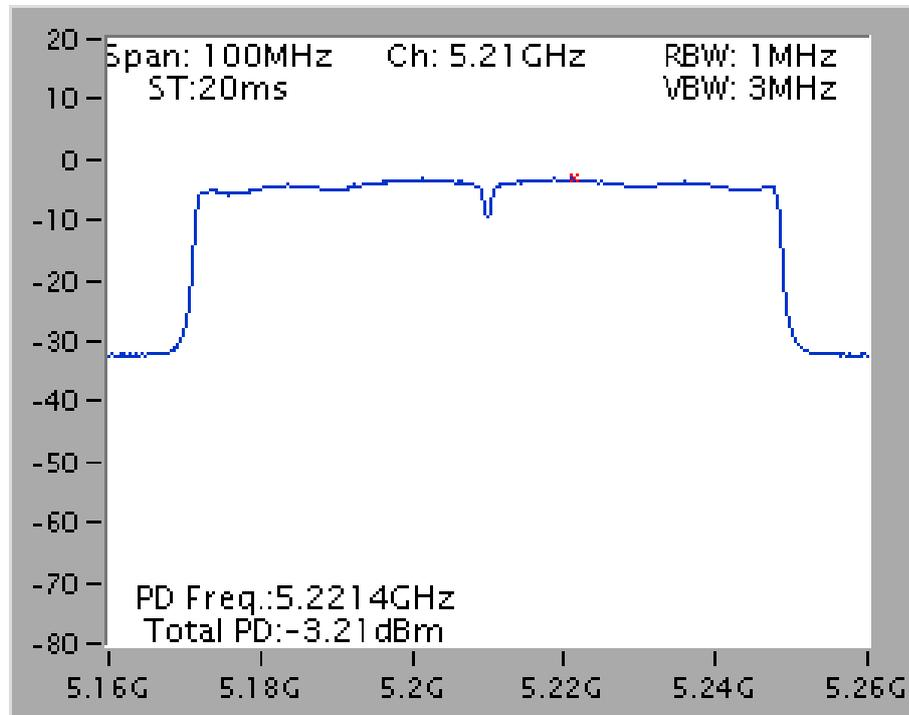
Power Density Plot on Configuration IEEE 802.11a / Ant. 3+ Ant. 4+ Ant. 5 / 5200 MHz
